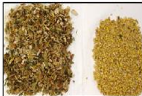
Figure 5. Example of separated stover and kernel fractions using the water separation technique.
