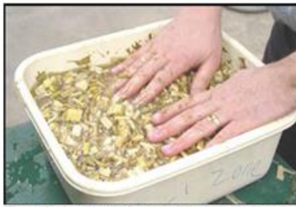
Figure 2. Gently agitating material to help the kernels sink to the bottom of the container.
